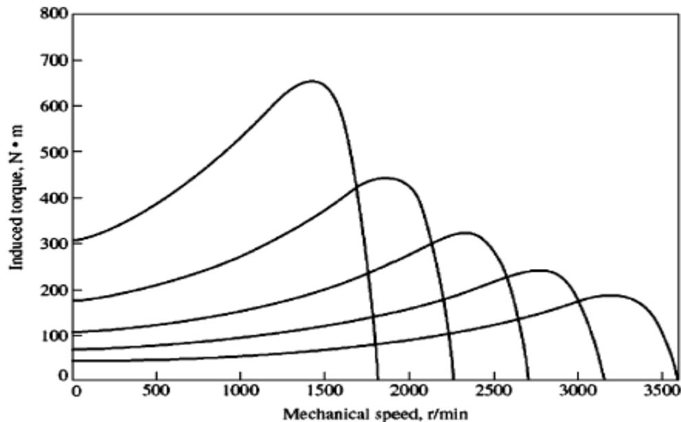
**Figure (b) : Variable-frequency speed control in an induction motor: The family of torque speed characteristic curves for speeds above base speed assuming that the line voltage is held constant.**
