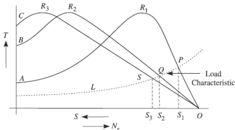
**Figure: Speed control of Slip ring Induction Motors by changing Rotor resistance
