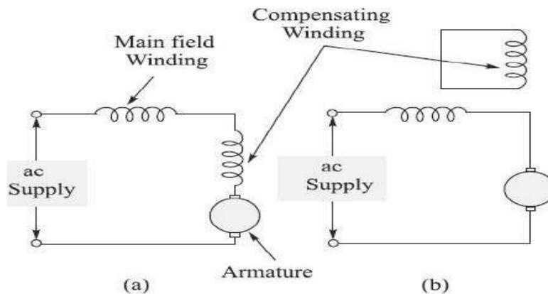
**Figure: Single-phase Series Motor with compensating winding**
