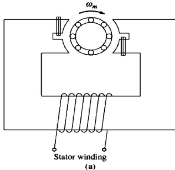
**Figure (a): A basic Shaded-Pole Induction Motor**
