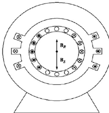
**Figure: The single-phase induction motor at starting conditions. The stator winding induces opposing voltages and currents into the rotor circuit resulting in a rotor magnetic field *lined* up with the stator magnetic field but in opposite direction as in a Transformer. But  $\tau_{\text{ind}} = 0$ .**
