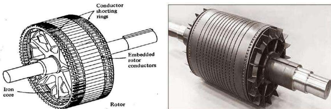
Figure :(a) Sketch of cage rotor. (b) A typical cage rotor.
