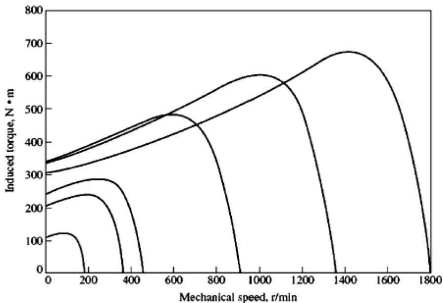
**Figure (a): Variable-frequency speed control in an induction motor: (a) The family of torque-speed characteristic curves for speeds below base speed. Assuming that the line voltage is derated linearly with frequency.**
