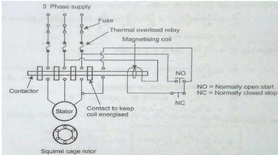
**Figure: Direct On Line Starter**
