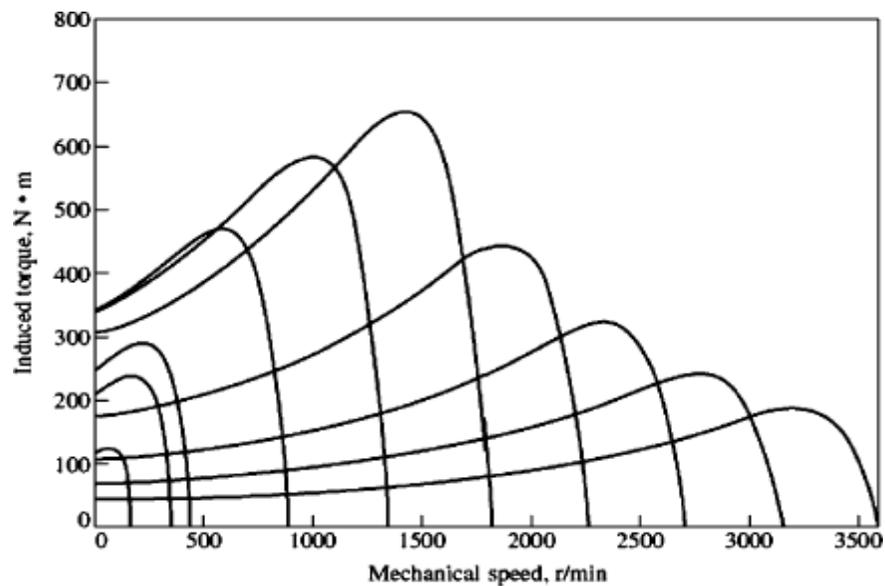
**(C) Variable-frequency speed control in an induction motor .The torque-speed characteristic curves for all frequencies.**
