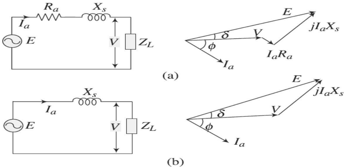
**Figure: (a) Equivalent circuit and phasor diagram of a synchronous generator
