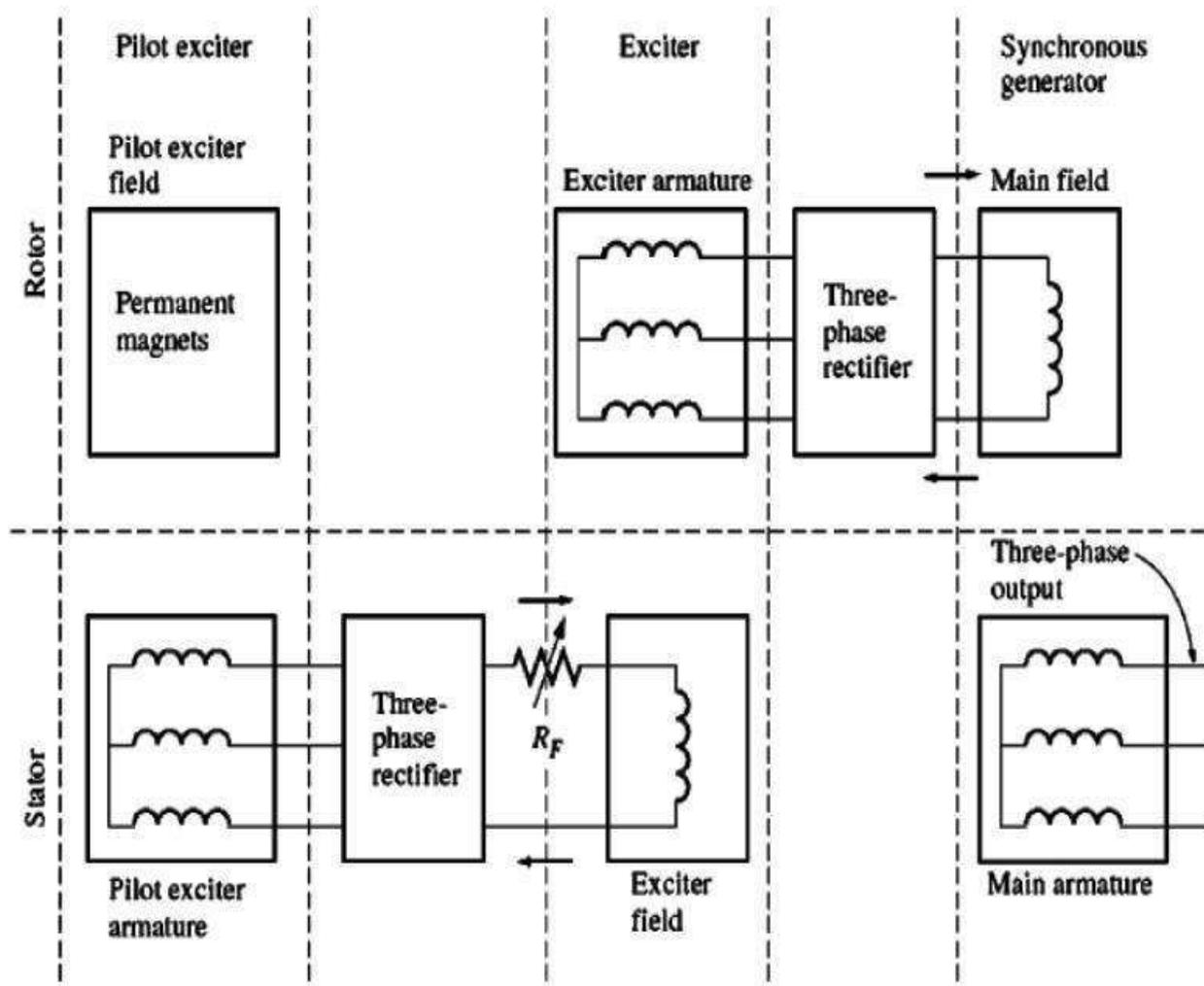
**Figure: A brushless excitation scheme that includes a pilot exciter. The permanent magnets of the pilot exciter produce the field current of the exciter which in turn produces the field current of the main machine.**
