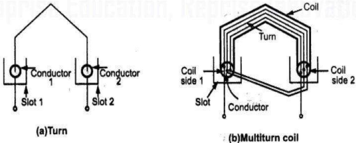
3) Coil: As there are number of turns, they are all grouped together to form a coil. Such a coil is called multiturn coil. A coil may consist of a single turn in which case it is called a single turn coil. Figure (b) above shows a multiturn coil.
