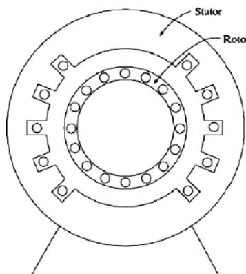
**Figure: Construction of a single-phase induction motor.**
