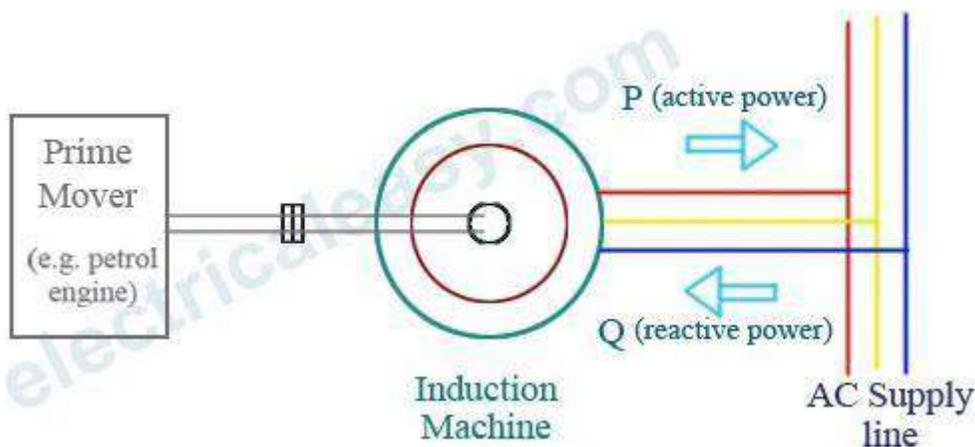
**Figure: Grid connected Induction Generator**
